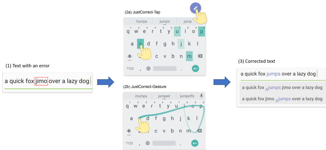
Figure 4.4: (1) The user enters a sentence with an error jimo using tap typing; (2) To correct jimo to jumps , they can either tap-type jumps and press the editing button (2a), or switch to gesture type jumps (2b). (3) JustCorrect then substitutes jimo with jumps . Two alternative correction options are also presented. The editing procedure involves no manual operations except entering the correct text.
